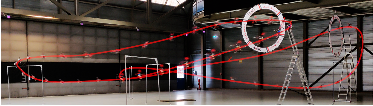
Figure 1: A time-optimal trajectory. This time-optimal flight path was computed using the proposed complementary progress constraints (CPC) and executed in a motion capture system, outperforming the best human expert.
